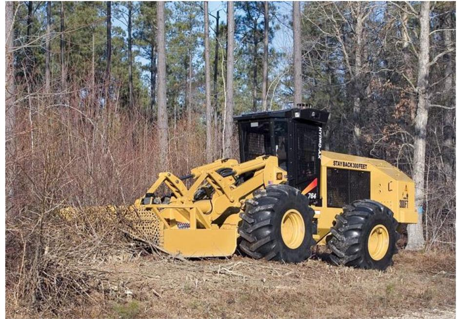
Hydro-axe equipment used for tree clearing
