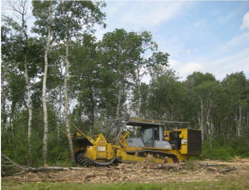
Drum-style mulcher used for tree clearing
